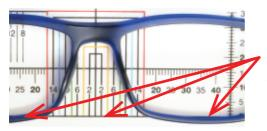
Place both lower inside rims on the horizontal line when lining up for lens measurement
