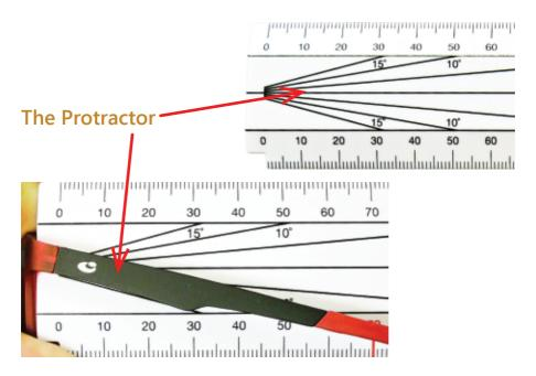
The protractor showing the pantoscopic angle of the temple
