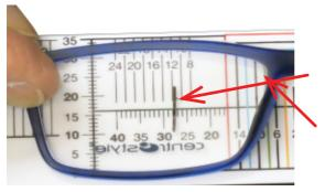
Easy measuring of monocular PD in conjunction with the alternated colour centration grid above
