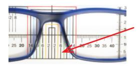
Alternate coloured grid lines at 2mm intervals makes layout easy for bridge centration and alignment
